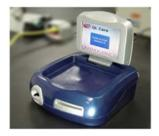
The QLCA represents a shift in the design POC analyzers. The QLCA is small, portable, stand-alone and completely automated point-of-care immunoanalyzer. The QLCA has successfully miniaturized lab test technology, and combined it with a simplified mechanical design and proprietary triggering mechanism.
